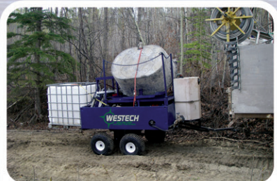
MOBILE GROUT PLANT
