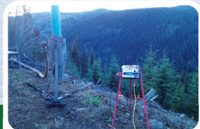
GAS MONITORING SYSTEM SENSORS
