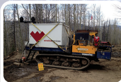
FLAT DECK SUPPORT UNIT
